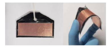
Electro-pneumatic pumps (EPPs) are micro air pumps that take advantage of recently developed dielectrophoretic liquid zipping technology. They can be made from any combination of insulating and conducting materials, allowing them to be extremely low-cost.
